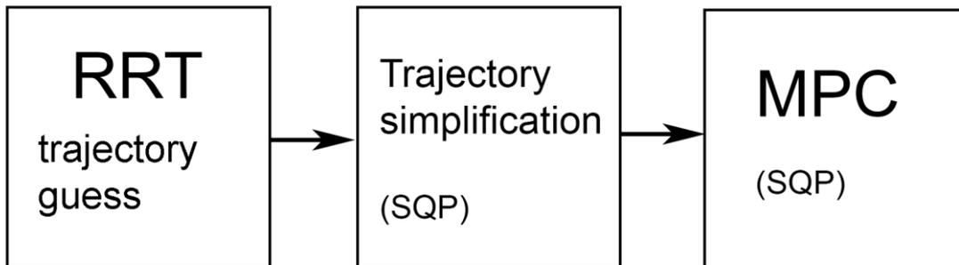
Figure 4.1: Flow of trajectory processing.
