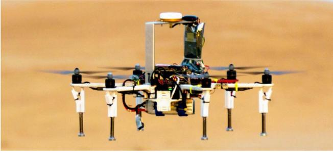
Fig. 7: MAV used in the experiments was based on DJI F550 hexacopter frame, Pixhawk stabilization board, and Intel NUC computer.
