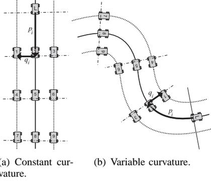
Fig. 1. Equivalent formations with time invariant Curvelinear coordinates  $p, q$  when following different trajectories.
